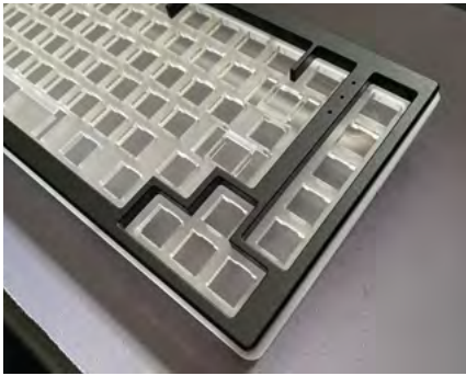
The switch plate and case combine to form the main structure and layout of the keyboard
