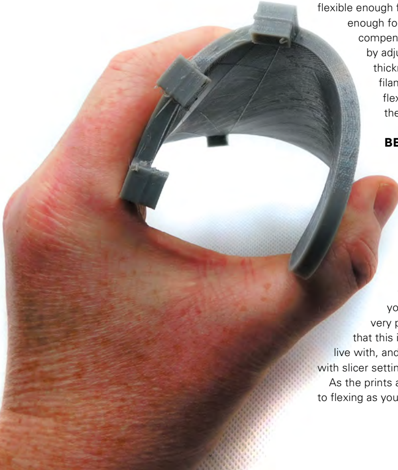
Right Two different designs of cable ties printed in TPU
