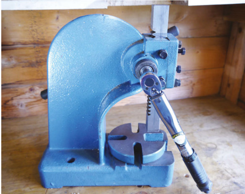
Figure 2 ♦ A simple modification allowing a torque wrench to be used as an alternate handle to deliver a repeatable force through the ram
