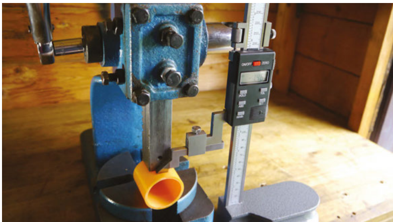
Figure 3 ♦ Using the torque wrench allows us to compare the strength and the strain in a 3D-printed part when under a known load. Using the height gauge allows us to measure the deflection of the 3D print
