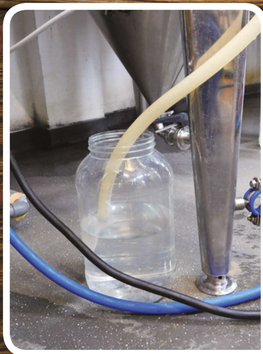
Above ⬆ Despite its size, brewery equipment isn't very different from what home brewers use – here's an airlock protecting the beer from oxygen
