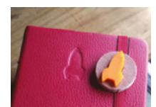
Figure 7 ♦ Using the press, we managed to emboss the shape from a 3D-printed object into a vinyl covered notebook
