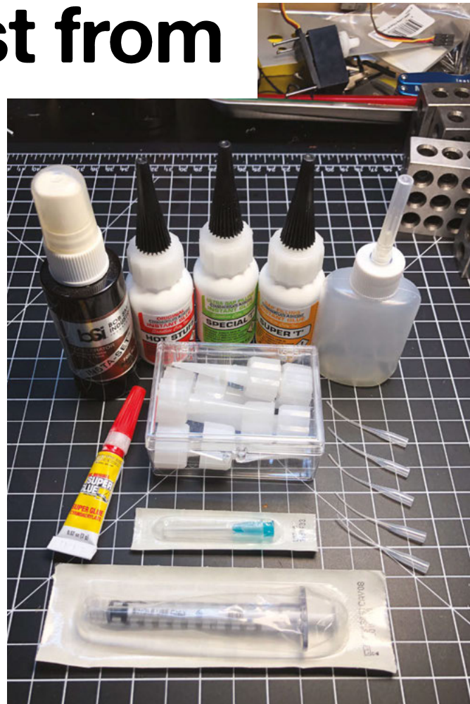
Above ♦ A selection of CA glues of different thicknesses and working times, accelerator, needle and Flexi-Tip applicators, and replacement 'snip-tip' nozzles
